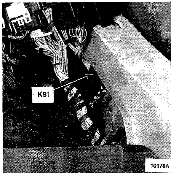
Figure 2- Below LH Side Of Rear Seat (Rear Power Distribution Box Removed)
