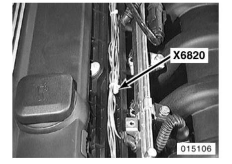
in injector valve rail
