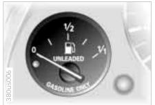
Please refuel early, since driving to the last drop of fuel can result in damage to the engine and/or catalytic converter.◀
