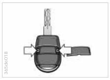
2 Loosen the two screws (arrows) and remove the cover.
