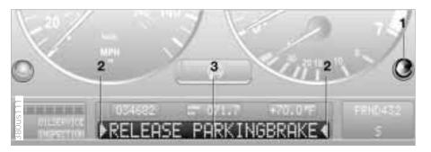
System malfunctions are reported in text form and alerts or warnings are each reported by a gong when the ignition key is in position 2.
