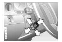
The steering wheel can be moved in any of four directions. Adjust by moving the control lever in the desired direction.
