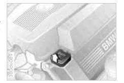
4 Start by connecting the jumper cable from the positive terminal of the support vehicle to the positive terminal connector located in your BMW's engine compartment. The cover of the auxiliary terminal for jump starting is marked with "Batt. +" (refer to the illustration). Remove by pulling tab. The illustration shows the auxiliary terminal for jump starting the BMW 740i/L as an example. For the BMW 750iL: Refer to "Engine compartment" on page 140
