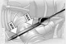
The oil volume between the two marks on the dipstick corresponds to approx. 1.1 US quarts (1 liter). Do not fill to beyond the upper mark on the dipstick. Excess oil will damage the engine.
