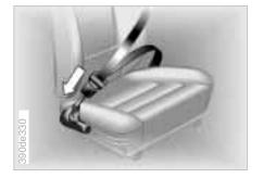
The safety belt tensioner responds to collisions by tightening the belts to ensure that occupants remain firmly positioned in their seats. A gas-pressure system retracts the buckle assembly to tension the shoulder and lap belts within fractions of a second. This reduces the tendency to slide under the lap belt.
