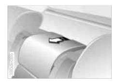
Stored between the rear seats. Pull the lever (arrow) and fold the cover forward.
