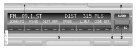
The onboard computer operates at ignition key positions 1 and 2.
