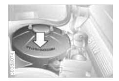
In the engine compartment, stamped on the right-hand strut dome (arrow) and on the upper edge of the instrument panel on the left side.
