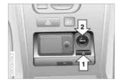
Push the lighter in (arrow 2). Remove as soon as the lighter jumps back out.
