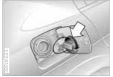
Open the filler cap carefully to prevent fuel from spraying out. Fuel spray may cause injury. Do not top off. Topping off may cause fuel spillage.
