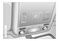
The reading lamps are located in the front near the interior lamp and in the rear. They can be switched on and off with the switch adjacent to each lamp.
