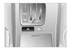
The push-button flashes rhythmically when the hazard flashers are on.
