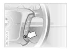
To activate and cancel the steering wheel heater, press button (arrow) with the ignition key in position 2.
