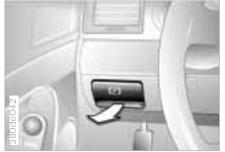
To release the brake, pull the handle. Please remember that the brakes disengage immediately.
