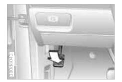
Depress the pedal. The "PARK BRAKE" (in Canada "P") indicator lamp in the instrument cluster comes on when the ignition key is in position 2.
