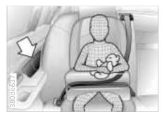
This is the right way a child should sit in a child restraint when rear side bags (arrow) are installed.
