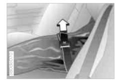
Secure the bag's contents by tightening down the strap at the buckle.
