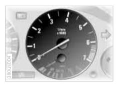
Never allow the engine to operate with the needle in the red overspeed zone of the gauge.
