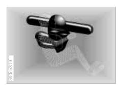
Deceleration sensors continuously monitor the physical forces acting upon the vehicle. In a severe frontal collision, the gas generators of the driver's airbag and the front passenger airbag are ignited. However, the passenger-side airbag is only triggered if an additional sensor has recognized that the passenger seat is occupied.
