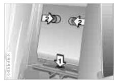
Press the release button (arrow 1) to unlock the cover panel in the luggage compartment.
