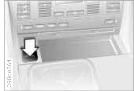
Press the cover panel for access (arrow), then push the lighter down.
