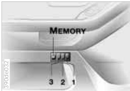
You can store and call up three different seat, exterior mirror and steering wheel positions. The illustration shows the buttons on the driver's door for making these position adjustments.
