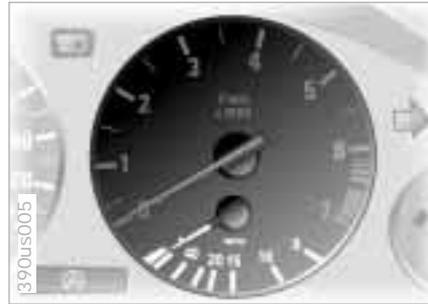
Indicates current fuel consumption in mpg (in liters per 100 km on Canadian vehicles). This instrument shows whether your current driving style is conducive to fuel economy with minimum exhaust emissions.
