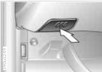
The Onboard Diagnostic (OBD) connector is located on the left of the driver's side at the bottom of the instrument panel and under a cover (arrow).
