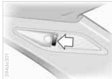
The reading lamps are located in the front near the interior lamp. There are also reading lamps in the rear. They can be switched on and off with the switch (arrow) adjacent to each lamp.
