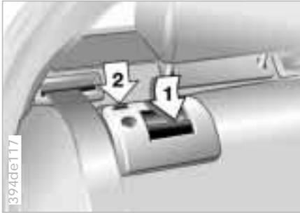
The backrest of the rear seat is divided into two portions, one-third and two-thirds of the seat respectively. For storing longer objects, you can fold down either side individually.
