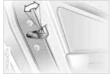
Insert the key into a rear door lock and turn it outward:
