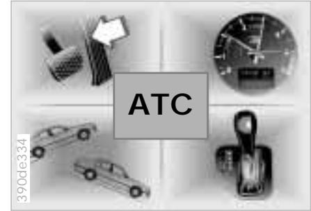
On vehicles with automatic transmission, Adaptive Transmission Control (ATC) uses a number of factors to calculate the gear which provides the maximum efficiency. In this process it monitors your personal driving style, the situation in which you are driving, the condition of the road and the traffic conditions.
