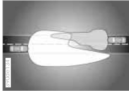
The xenon lamps light up the side and front areas of the vehicle with significantly more brightness and uniformity than the traditional halogen lamps.
