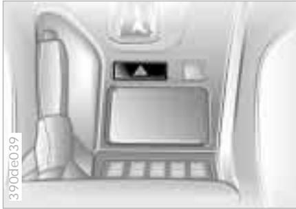
The button flashes rhythmically when the hazard warning flashers are on.
