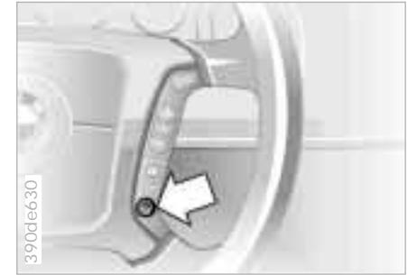
To activate and cancel the steering wheel heater, press the button (arrow) with the ignition key in position 2.
