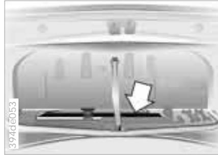
The hazard warning triangle is quickly available, stored in the onboard tool kit mounted on the inside of the luggage compartment lid (tailgate). To open the container, loosen the wing screw.
