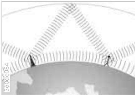
AM provides substantially longer reception ranges than FM. AM broadcast signals, propagated at ground level in the form of surface waves, are also reflected from the ionosphere as atmospheric waves.
