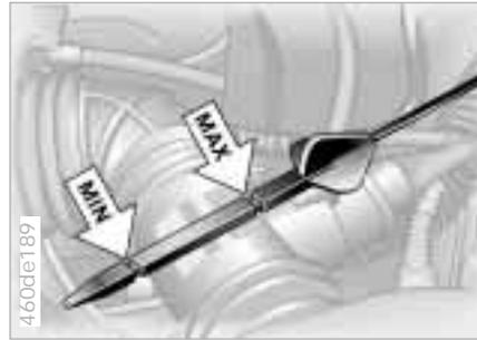
The oil volume between the two marks on the dipstick corresponds to approx. 1.1 US quarts (1 liter). Do not fill beyond the upper mark on the dipstick. Excess oil will damage the engine.
