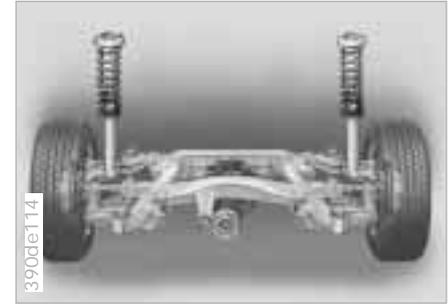
The control arms on the patented integrated aluminum rear axle assembly are not mounted directly on the body. They are mounted elastically on a chassis sub-frame which is joined in turn with elasticity to the vehicle body. The resulting double elastic suspension system effectively absorbs the forces resulting from bumps and road surface irregularities.
