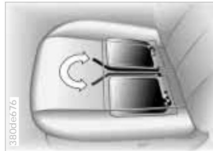
BMW seats are configured for your orthopedic well-being. The active seat is an engineering enhancement of BMW's seats, designed to ensure less fatigue during extended trips while sitting with little movement. The seat is no longer a passive element between the road, the running gear and the passenger. Instead, it creates minor and imperceptible shifts in your weight by an active change in the contour of the seat surface. The basic seat position is not changed as this occurs.
