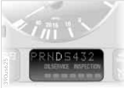
The automatic transmission of your BMW is equipped with Adaptive Transmission Control (ATC), a system which reacts with precision to your individual driving style and the driving conditions. To achieve this, different driving programs are automatically engaged.
