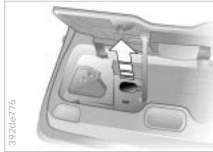
2. Release the two quick-release fasteners of the cover for the onboard tool kit in the tailgate. Raise the cover
