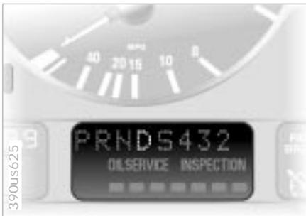
The automatic transmission of your BMW is equipped with Adaptive Transmission Control (ATC), a system which reacts with precision to your individual driving style and vehicle operating conditions. ATC operates by automatically selecting from among a range of available control programs.
