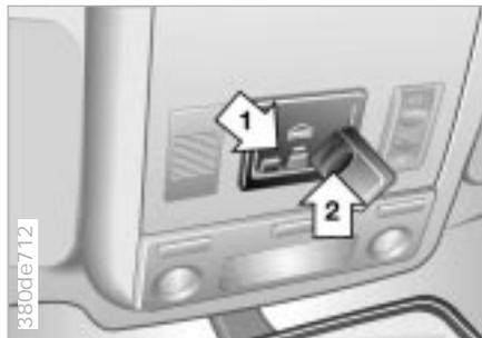
3. Hold the original hand-held transmitter at the receiver 3 a maximum of 2 in (5 cm) away
