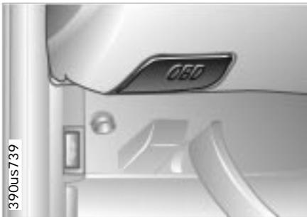
The Onboard Diagnostic (OBD) interface socket is located on the left of the driver's side at the bottom of the instrument panel and under a cover. The cover has the letters "OBD" on it.
