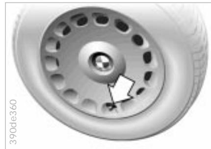
4. Wheels with adapter\*: position the lug bolt adapter on the lug bolt cover. Then apply the lug wrench and turn it to the left (refer to the illustration)
