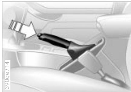
The parking brake is primarily designed to prevent the vehicle from rolling while parked. It operates on the rear wheels.
