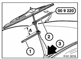
If the contact angle is incorrect, the wiper arm must be turned into correct position using two special tools 00 9 220.
