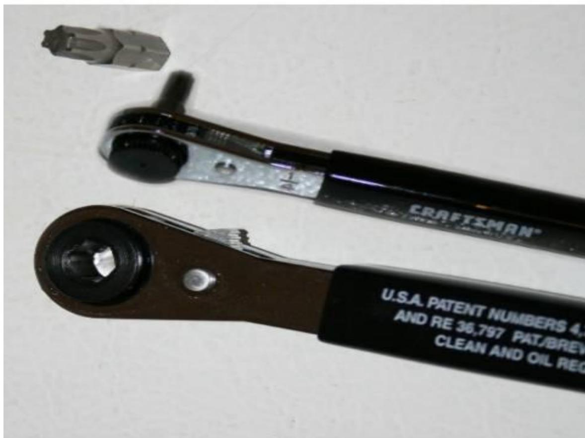
You have to have a tool like this; Joe C uses an HVAC wrench. As long as it is thin and ratchets w/magnetic bit holder, it will work.
