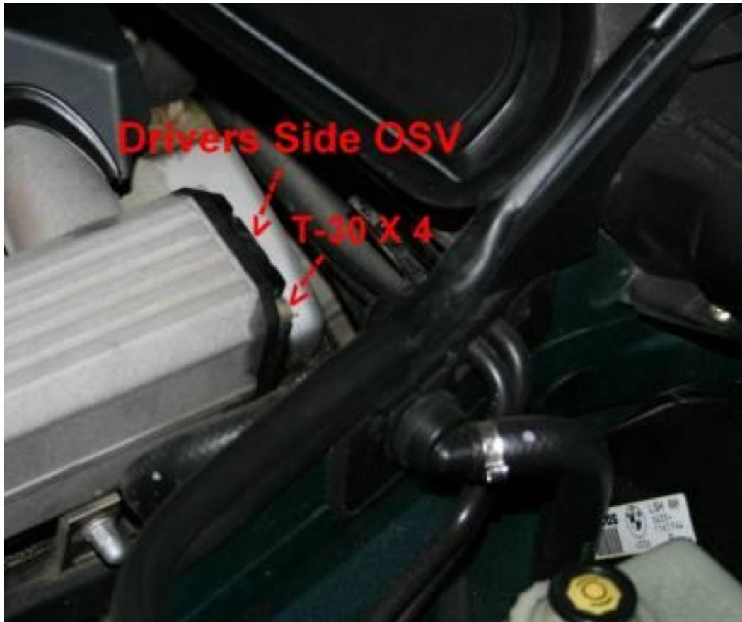
Remove the four torx bolts (which do not strip, unlike the V8's), bottom screws first so top will hold valve in place. Now pry the valve loose in case it is stuck to the intake, the valve will stay attached by #5 the rubber boot to the valve cover. Now reach down and remove the valve from the boot, if you tear the boot, ok, it needs replacing anyway. Once you get the OSV cover out, you can reach down and remove the boot from the valve cover nipple.
