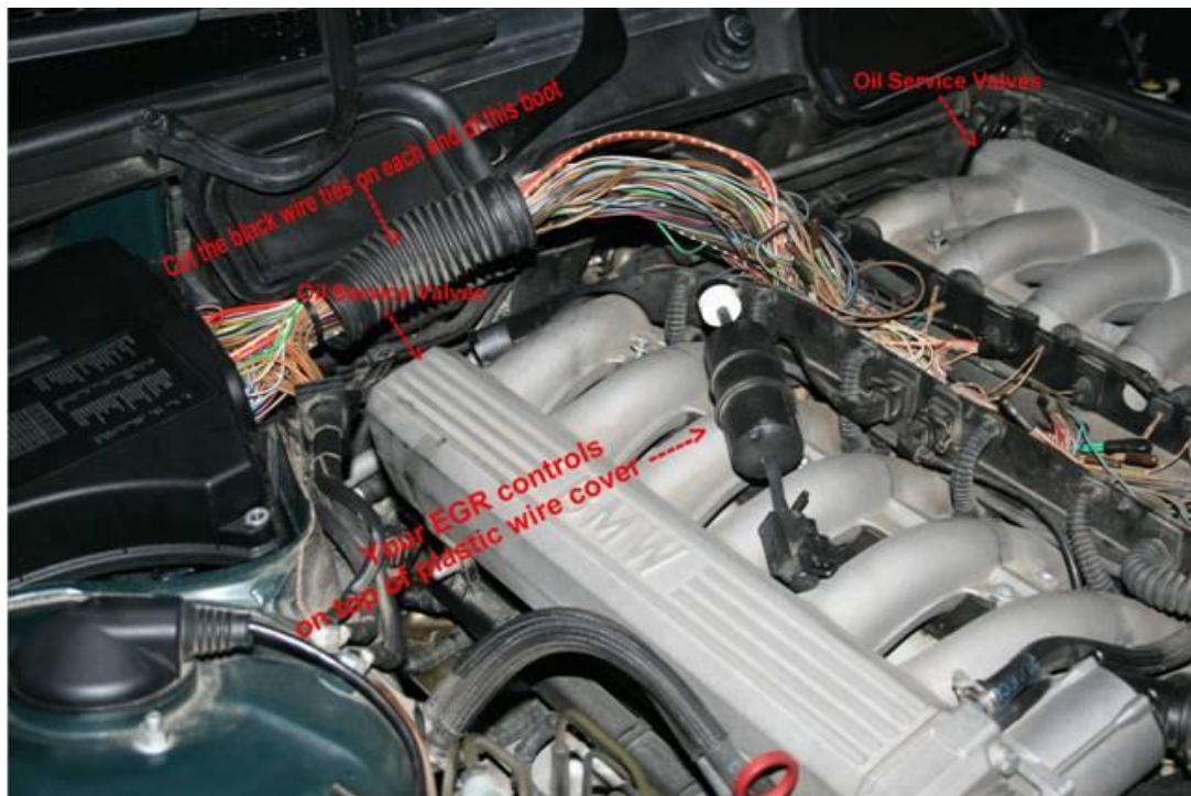
Cut the two zip straps that hold the rubber boot to the plastic on each end. (see picture)
