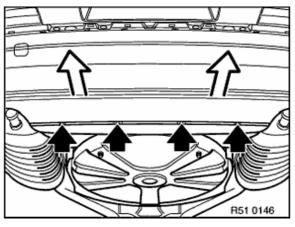
Unclip bumper from underside of guide.
