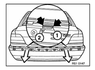
Pull bumper slightly backwards and remove fillister head screw out of bore (2) at oblique angle using bar magnet.
