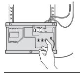
The garage door opener should now recognize the HomeLink Wireless Control System. The remaining two buttons may now be trained if this has not previously been done. Refer to the Programming portion of this text. The HomeLink Wireless Control System (once programmed) or the original handheld transmitter may be used to activate the garage door. In the event that there are still difficulties in programming the HomeLink Wireless Control System, please visit our Web site, www.homelink.com.
