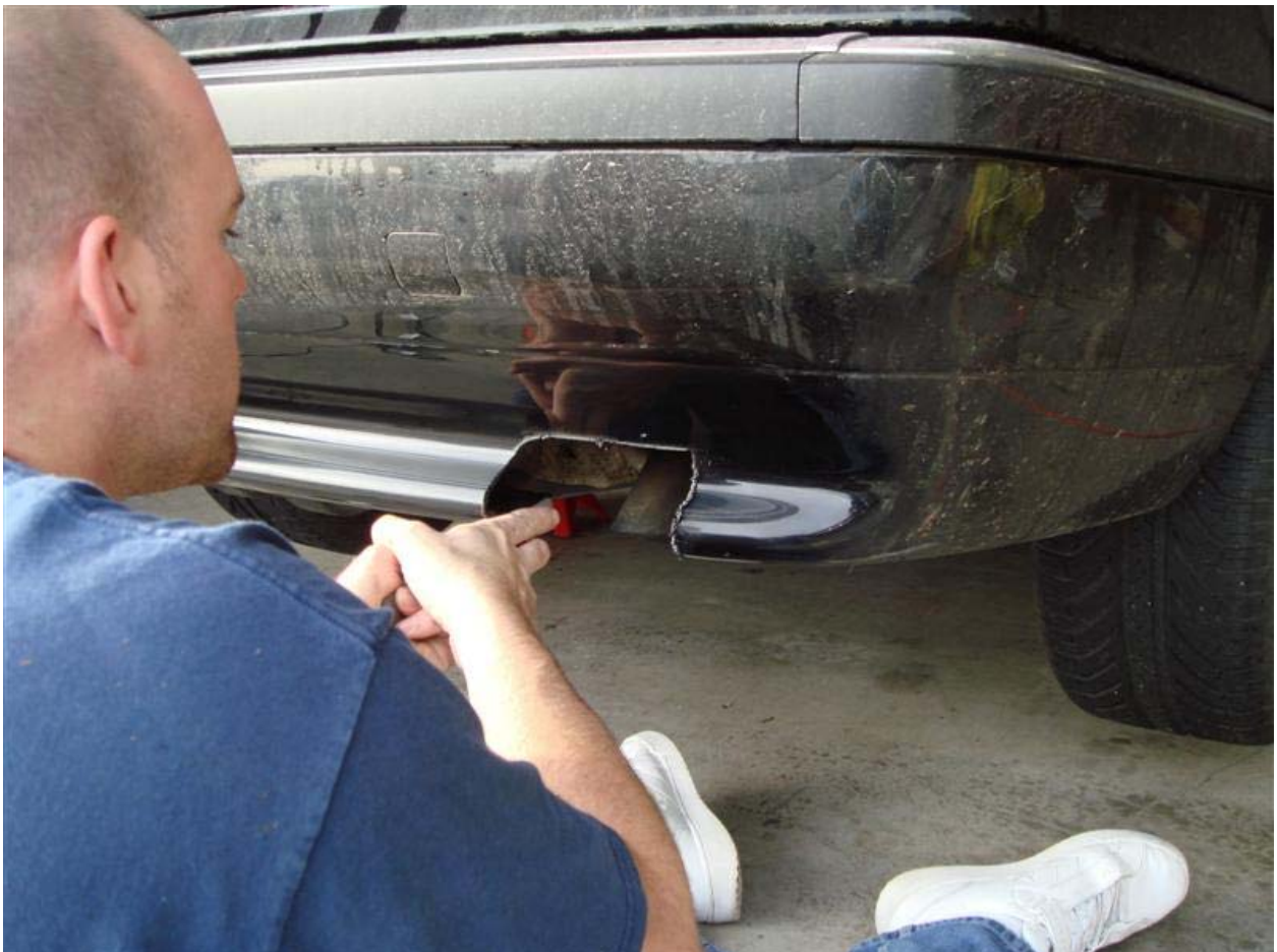
Image 6: Filing away slag and imperfections.
