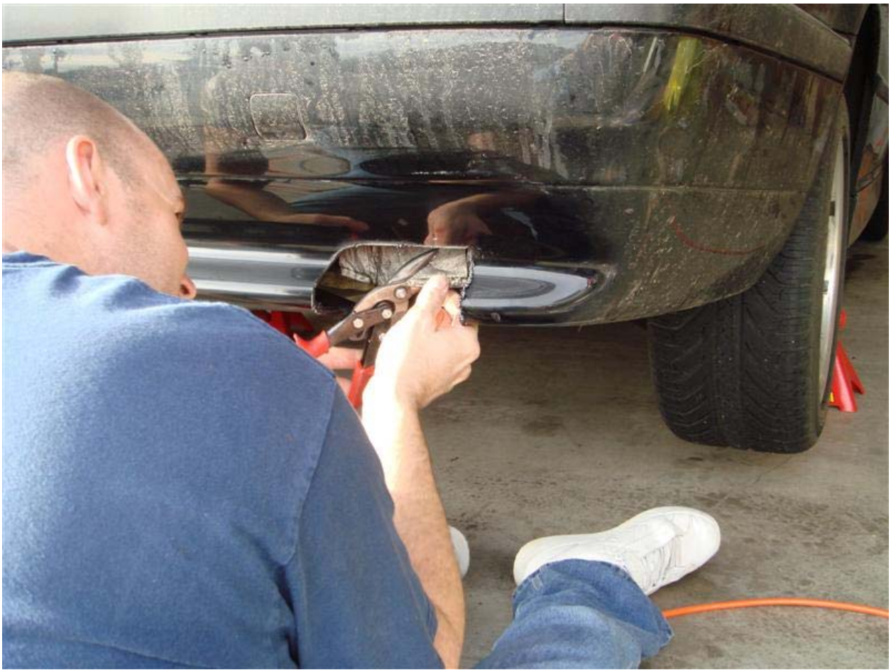
Image 3: Removing heat shield material.
