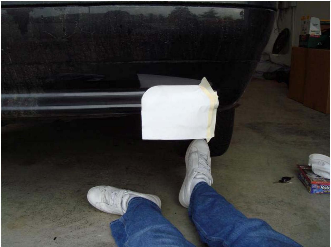
Image 4: Placing the template for the second cut.
